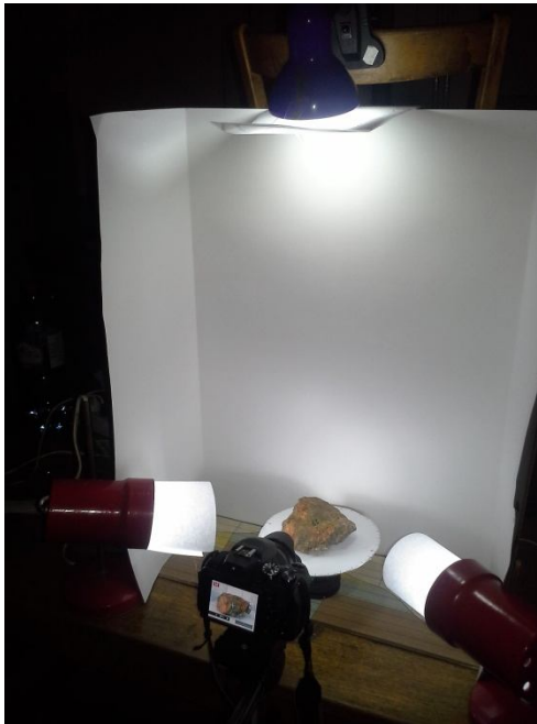
Fig. 2 Final setup with diffuse white lights, a tripod and a turning table for the sample.
