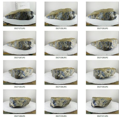
Fig. 3 Examples of photos taken for the sodalite sample. 12 photos from a total of 256 photos.
